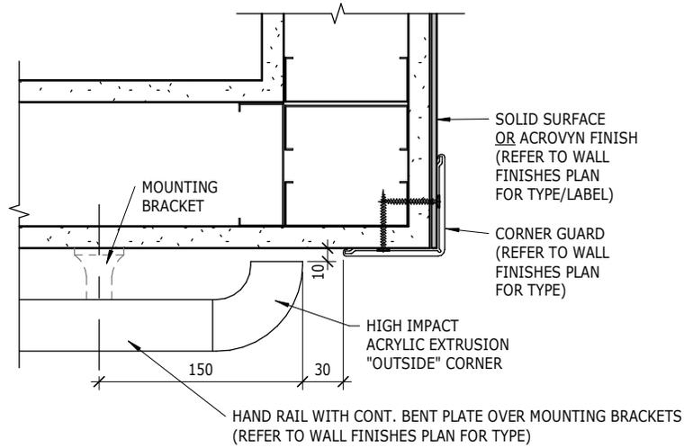
TYPICAL PLAN DETAIL OF HAND RAIL, SHEET WALL PROTECTION AND CORNER GUARD
