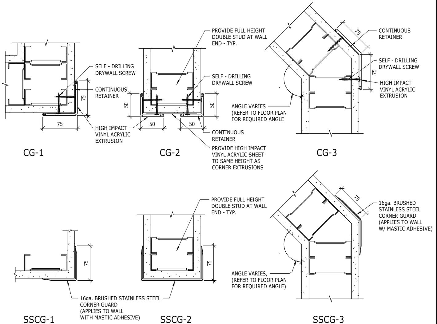
**NOTE:** CORNER GUARDS IN PUBLIC/PATIENT AREAS TO BE SECURED WITH TAMPER-RESISTANT SCREWS AND CONT. TAMPER-RESISTANT SEALANT AROUND EACH UNIT.
