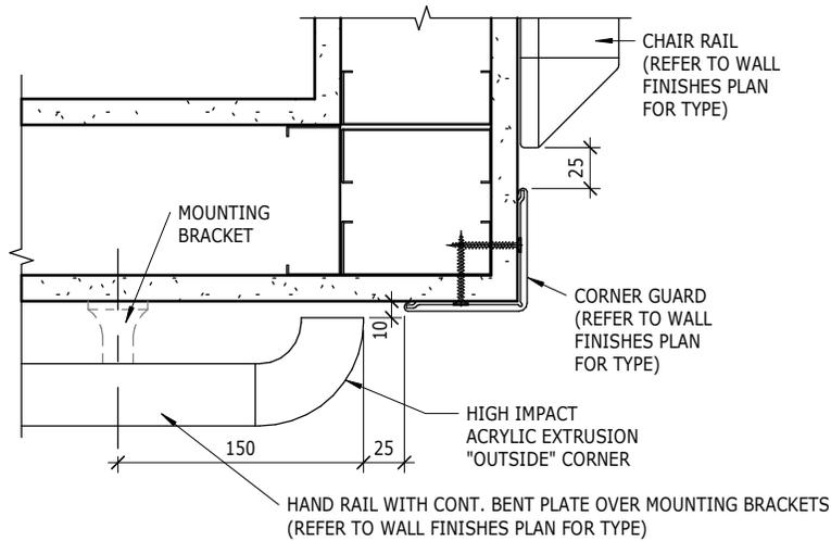
TYPICAL PLAN DETAIL OF HAND RAIL, CHAIR RAIL AND CORNER GUARD
