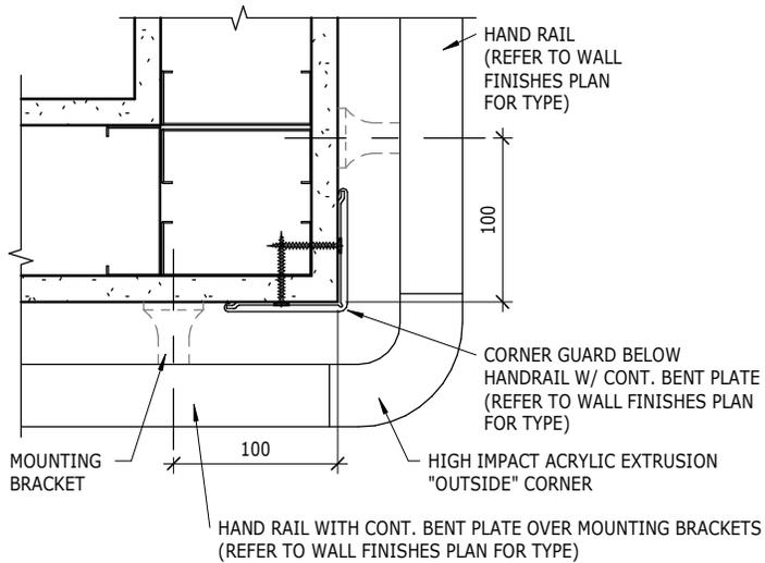
TYPICAL PLAN DETAIL OF HAND RAIL AND CORNER GUARD
