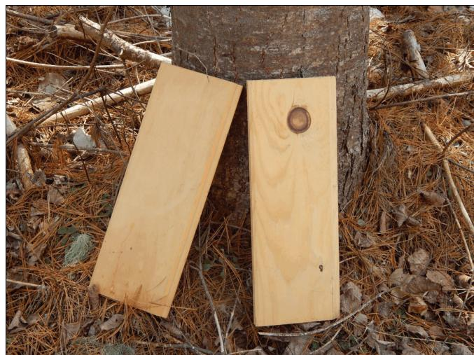
Knots are defects which can tarnish the look of the wood and decrease its strength and load-bearing capabilities. As a rule, the larger the knot, the bigger the defect in the wood and thus, the lower the value of the wood. This also applies to wood with multiple small knots.
