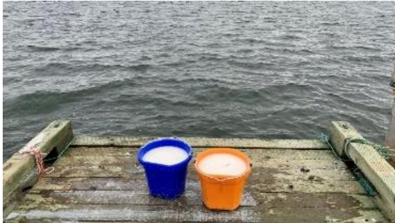
Figure 3. Hydrated lime (4%) and brine (30% salt) mixture prepared for the treatment trial; 600g of hydrated lime and 4050 grams of salt in 15L of seawater.
